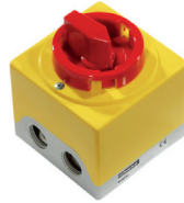
Safety start/stop switch to stop the fan before any maintenance work. Compliant with IEC 947-3 standard. Protection IP-65
